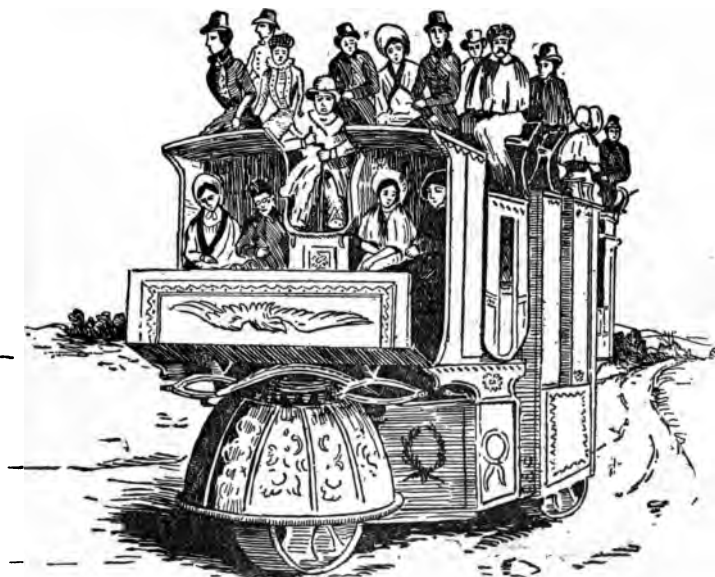
FIG. 9.—Church's Three-wheel Coach (1833), drawn from an old woodcut, showing forward spring wheel mounted on the steering pivot.
